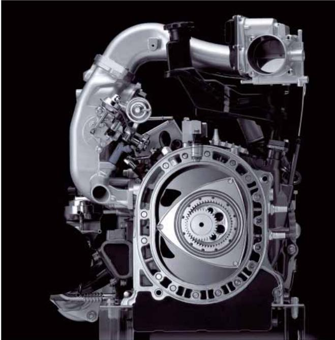
The other key characteristic of hydrogen is that it produces less energy at equivalent volumes when combusted, because it has a lower density than petrol. The low density of hydrogen - injected in its gaseous state - means that at the quantity required for combustion, it would occupy 29.5 % of the volume of the combustion chamber, compared to a mere 1.7 % for petrol. The result would thus be a reduced quantity of injected air, resulting in incomplete combustion and reduced power.
